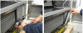
Remove the closing panel screws. Remove the closing panel. Remove the electrical panel locking screw. Move the electrical panel box along the slide.
