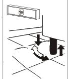
Level the appliance by means of adjustable feet.
