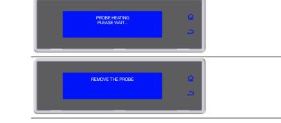
In the event that the temperature read by the needle core sensor is not negative, the function will not be activated.
