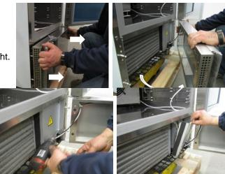
Remove the electrical panel locking screw. Move the electrical panel box along the slide.
