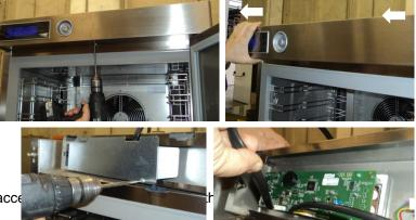
Undo the guard screws and remove the cover to acce encoder.
