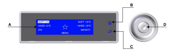
A-Display: Displays all the information relative to the menus on the board and the application in progress.
